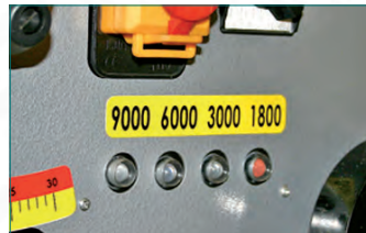
Light display for easy-to-read speed indicator
