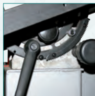
Rack and pinion 45° table tilt
