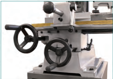
Multi-height, depth table adjustment
