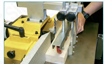
Independently micro-adjustable outfeed fence
