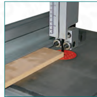
Auxiliary fence for cutting thinner materials
