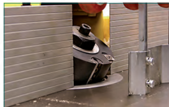
Spindle tilt from -10° to +30°
