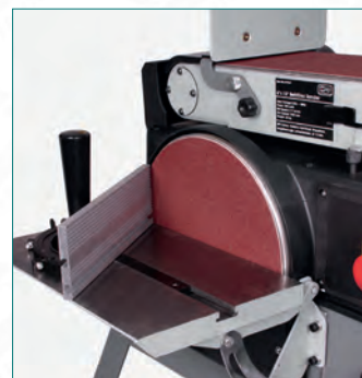
Cast-iron machined tilting table with cast mitre fence
