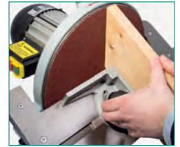
Cast iron machined tilting table with T-Slot
