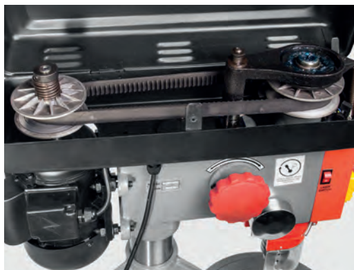
Easy infinitely variable speed control
