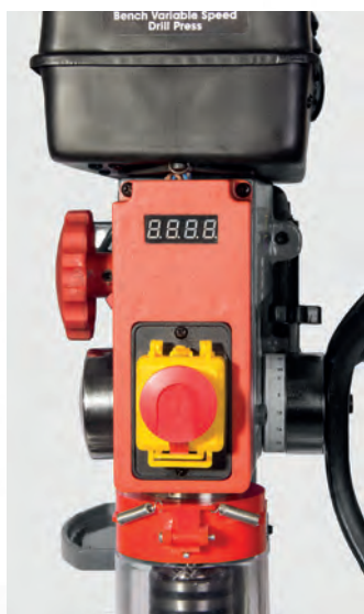
LCD digital speed display
