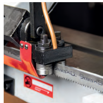
Blade guide rollers with integrated lubrication pipe
