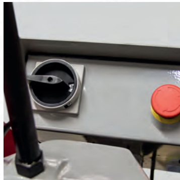
Clear control with NVR switch
