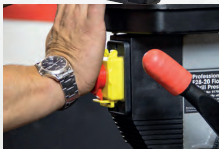
Magnetic NVR switch for added safety
