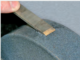
8" slow speed wet grinding wheel - perfect for a finer finish (07576)
