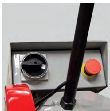
Clear control with NVR switch included
