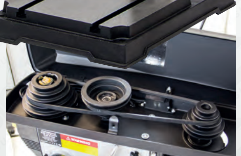
Quick and simple 'easy-lock' motor speed adjustment
