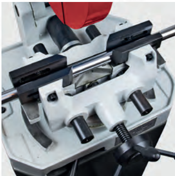
Twin vice - centralises the workpiece
