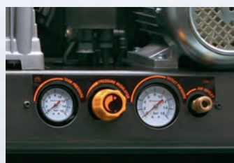
Built-in pressure regulator with large adjustment knob and easy-to-read dials
